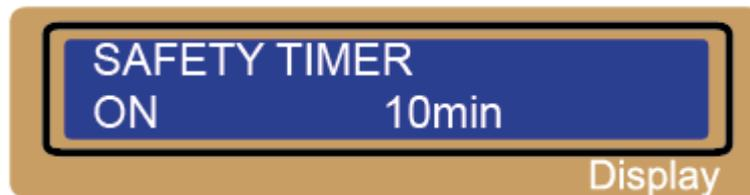
When you start a charge process, the integral safety timer automatically starts running at the same time. This is programmed to prevent overcharge the battery if it proves to be faulty, or if the termination circuit cannot detect the battery full. The value for the safety timer should be generous enough to allow a full charge of the battery.
