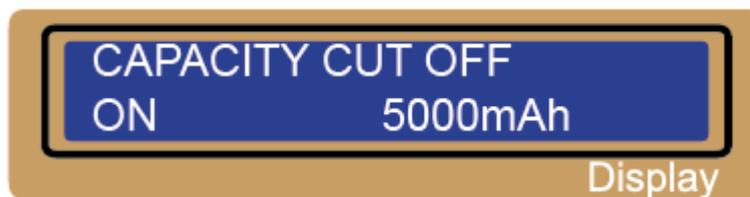
This option sets the maximum charge capacity that will be supplied to the battery during charge. If the delta-peak voltage is not detected nor the safety timer expired by any reason, this feature will automatically stop the process at the selected capacity value.
