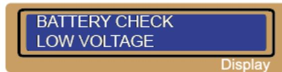
The processor detects an under voltage.
