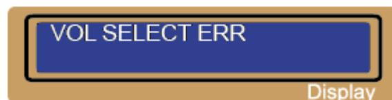
The voltage of Lithium battery pack was selected incorrectly. Verify the voltage of battery pack carefully.
