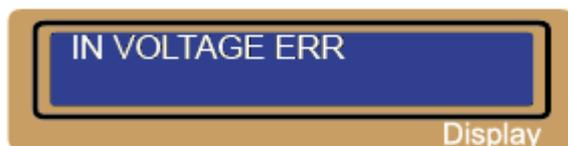
The voltage of input power lowers the limit
