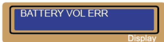
The voltage of one of the cell in the LiPoly battery pack raised over the limit.
