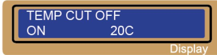
An optional feature using temperature probe contacting the surface of battery, the temperature cut-off can be on or off. If it is on, set the maximum temperature at which the charger should allow battery to reach during charge. Once a battery reaches this temperature during charge, the process will be terminated to protect the battery.
