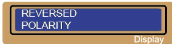
The output is connected to a battery with incorrect polarity
