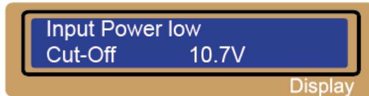
This program monitors the voltage of input battery. If the voltage drops below the value you set the operation forcibly terminated to protect the input battery.
