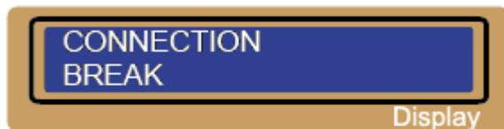
This will be displayed in case of detecting an interruption of the connection between battery and output
