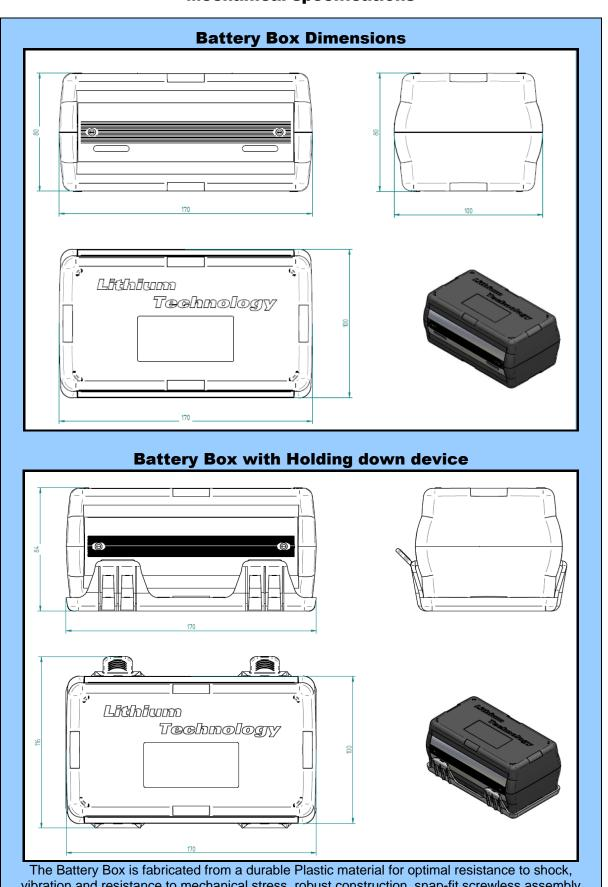
vibration and resistance to mechanical stress. robust construction, snap-fit screwless assembly
