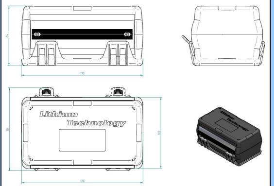
The battery box is fabricated from a durable plastic material for optimal resistance to shock, vibration and resistance to mechanical stress. Robust construction, snap-fit screwless assembly.
