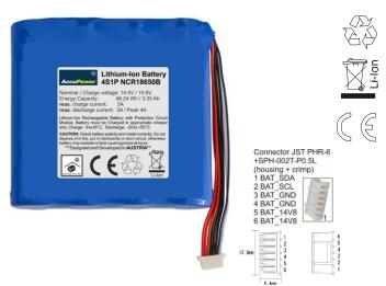
Lithium-Battery Pack with protection electronics (PCM single cells monitoring), protects the battery against overcharge, deep discharge and short circuit, Implemented cell balancing, and Gas Gauge with SM Bus Interface
