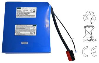
Lithium-Battery Pack with protection electronics (BMS single cells monitoring), protects the battery against overcharge, deep discharge and short circuit, Implemented cell balancing, with I2C-interface for service purposes (number of cycles, capacity, temperature, etc.)
