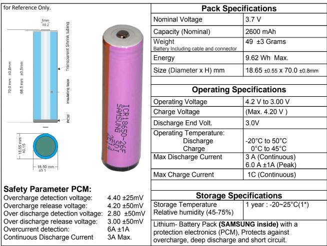
Note (1): If the cell is kept as ex-factory status (50% of charge), the capacity recovery rate is more than 80%.
